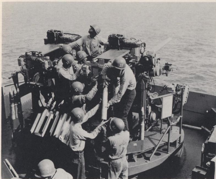
3 INCH 50 CALIBER ANTI-AIRCRAFT GUNS
