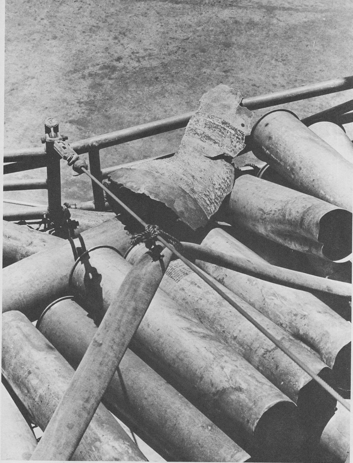
Photo taken October 3, 1972 showing the "Basket" attached to the front of No. 2 turret. The "Basket" catches empty brass ejected from the turret. Official U.S.N. Photo.
