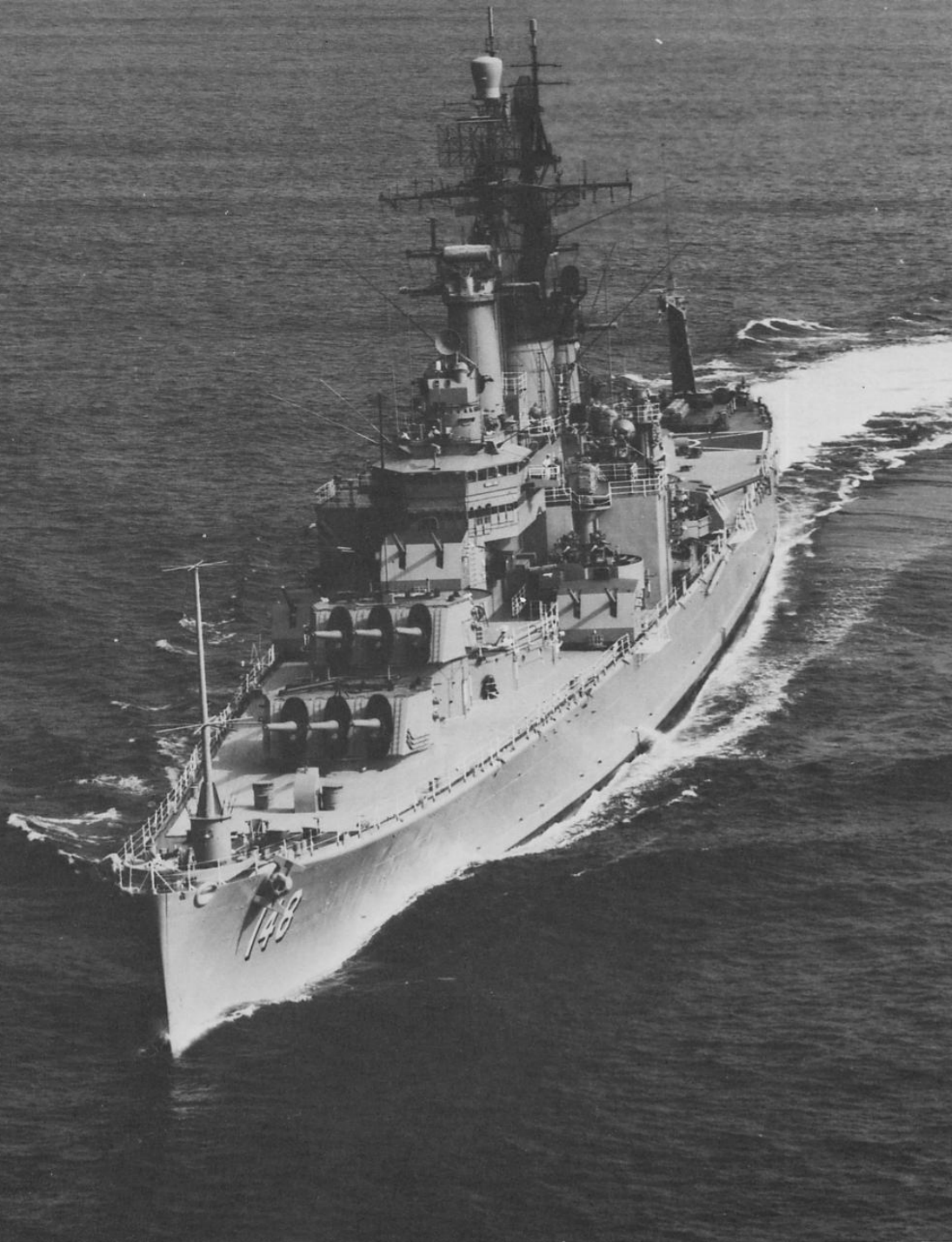
Opposite page: CA-148 after modification to flagship. Note extended superstructure, removal of various 3" guns and addition of antenna on forecastle. Official U.S.N. Photo. Above: The U.S.S. NEWPORT NEWS under way off the coast of Oahu, Hawaii, September 25, 1967. Official U.S.N. Photo.
