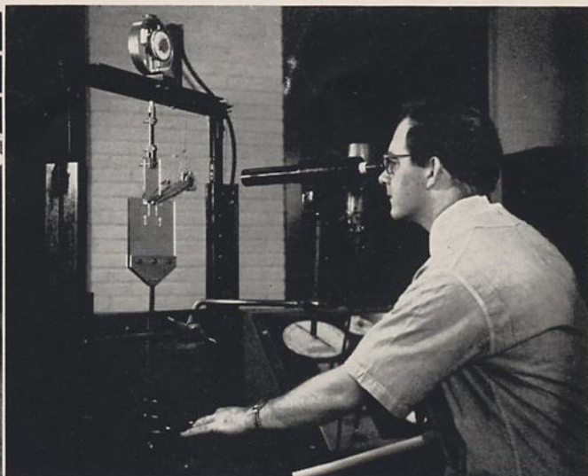
Roscoe Meadows, Jr., operating an Optical Interferometer Type of Lateral Strain Gage.
